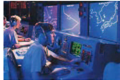
The Vincennes ’ CIC (Combat Information Center). Note the three large 42 x 42” displays and the smaller 12” displays below
